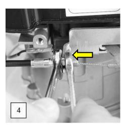
2.30 Check the cable adjustment has worked by starting the mower. If the mower still fails to start, re-adjust until the lawnmower starts.
